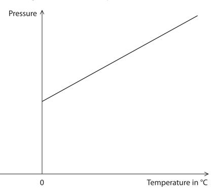
(i) Describe how the graph can be used to show that there is a minimum value of temperature, known as absolute zero.
